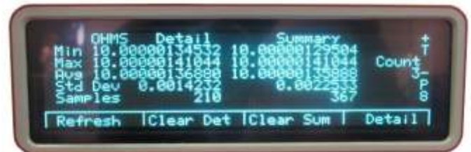
Examples of Actual 6622A Display Pictures Taken at Trade Shows - Note Std Dev is in ppm showing ppb performance!
