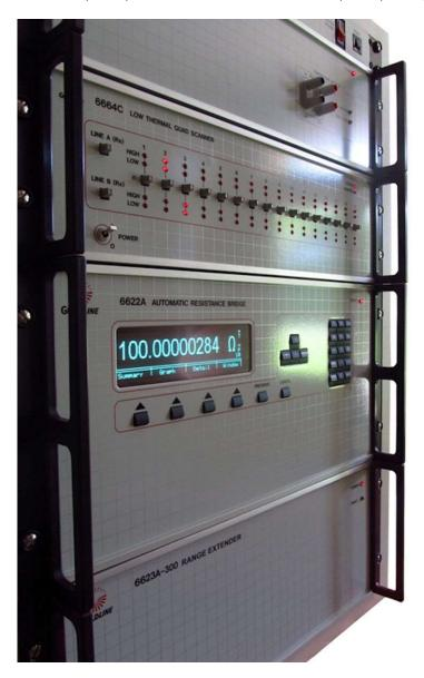
A 6625A rack that also includes a power module, rear door, dual fans, and a high quality grounding plane included!
