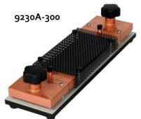
For models from 300 A to 500 A, Guildline utilizes a higher power copper current input terminal, with a single current terminal connection. The number one selling model in this design is our 9230A-300. Like all Guildline Shunts, notice the circular current connections and precision cut-outs to channel the current allowing for the best in repeatability and stability for current measurements.
