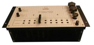
terminal shunt. The design optimizes a number of important factors such as the effects of self-heating, temperature coefficient, size, weight, ease of operation and total measuring range. They provide wide range precise current measuring capability when used with a potentiometer or digital voltmeter as a readout.
